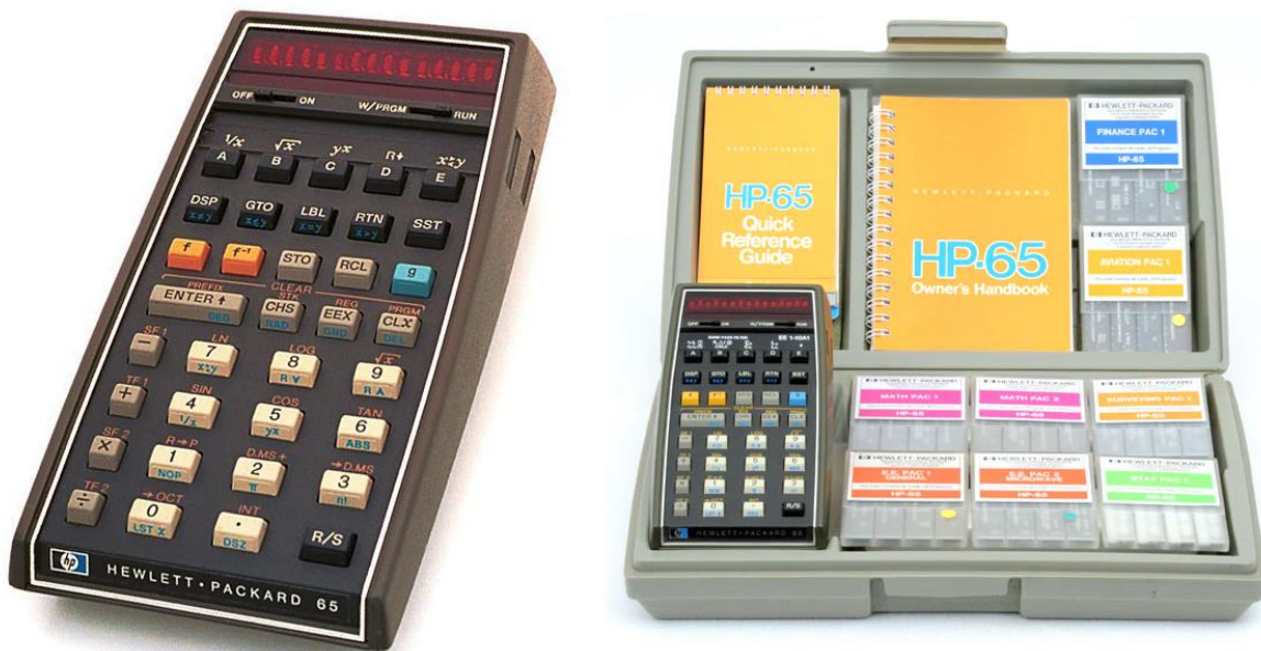
Fig. 2. HP-65 – the first programmable handheld calculator in space used in the 1975 Apollo-Soyuz Test Project
