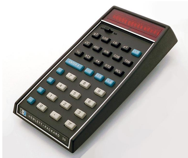
Fig. 1. HP-35 introduced in 1972 was the first world's scientific calculator. It used the postfix notation. Attribution: Hweih [CC BY-SA 3.0 ( http://creativecommons.org/licenses/by-sa/3.0/ )]
