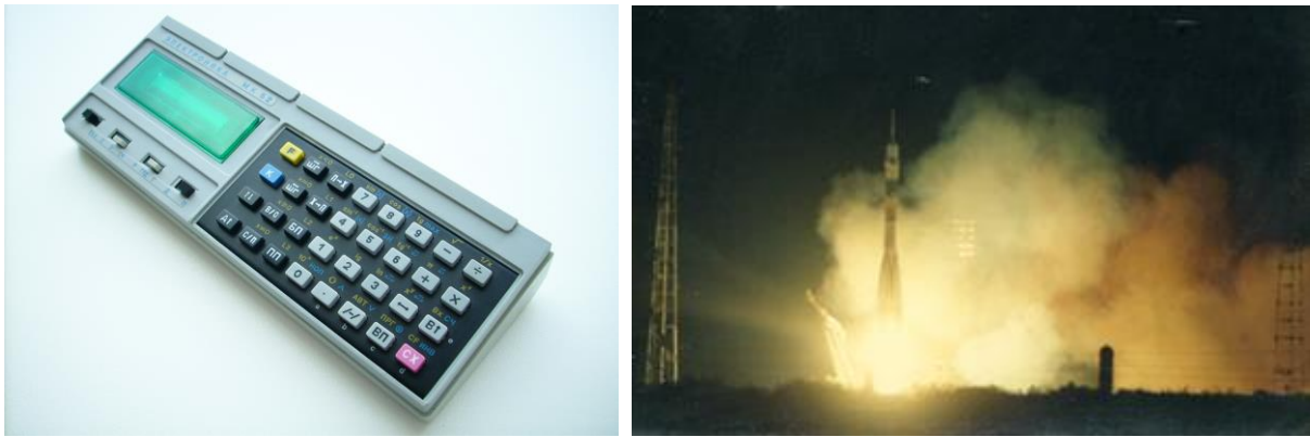
Fig. 4. Elektronika MK-52. The first Soviet programmable postfix calculator used in space flow on the “Soyuz TM-7” mission.
